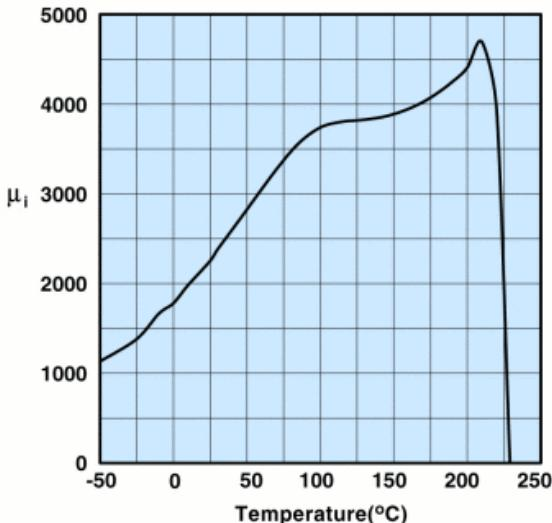
Measured on an 18/10/6mm toroid at 100kHz.
