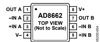
Figure 4. AD8662, 8-Lead MSOP (RM-8)
