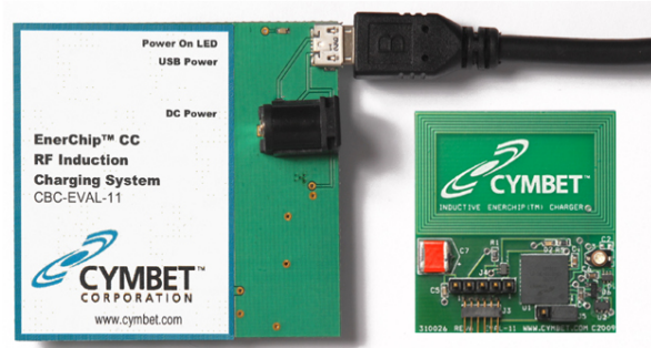
Figure 2: CBC-EVAL-11 Evaluation Kit. PCB colors may be green or red.
