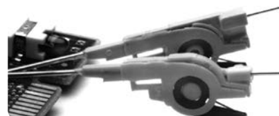
Extremely small-sized clips for probing PQFP and SOIC SMT packages.
