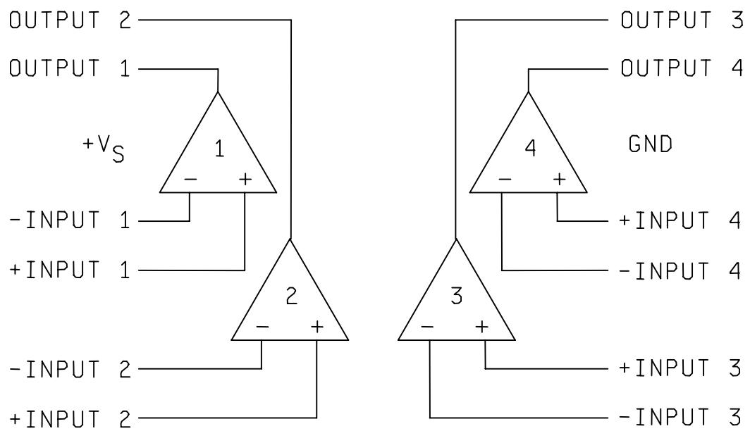
FIGURE 2. Logic diagram.
