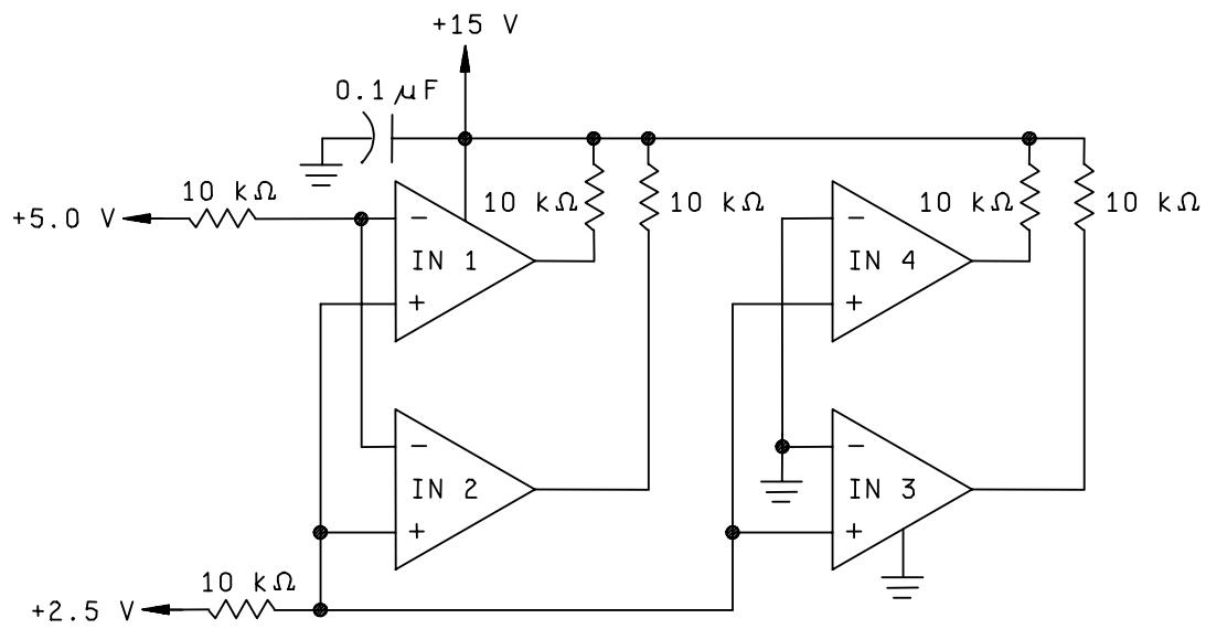
FIGURE 3. Radiation exposure circuit.
