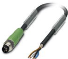
Sensor/actuator cable, 4-position, PUR halogen-free, black-gray RAL 7021, shielded, Plug straight M8, on free cable end, cable length: 3 m
