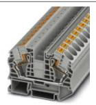
Feed-through terminal block, Connection method: Push-in connection, Cross section: 0.5 mm<sup>2</sup> - 25 mm<sup>2</sup>, AWG: 20 - 4, Width: 12.2 mm, Color: orange, Mounting type: NS 35/7,5, NS 35/15
