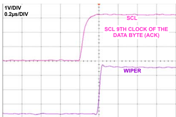
FIGURE 21. WIPER LARGE SIGNAL SETTLING TIME
