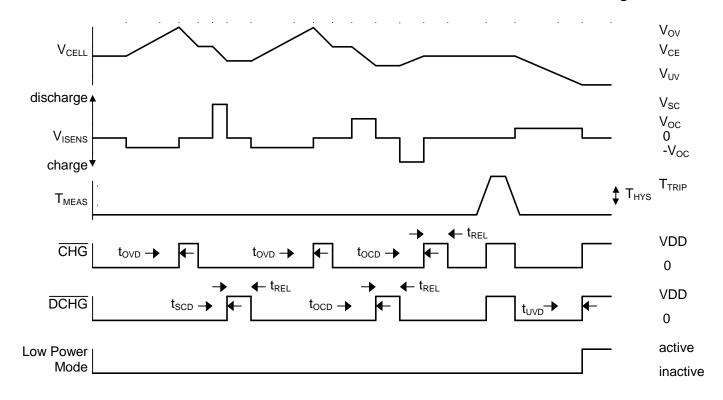
**Summary.** All of the protection conditions described above are OR'ed together to affect the  $\overline{\text{CHG}}$  and  $\overline{\text{DCHG}}$  outputs. Taking the OV, UV and OT bits from the Status Register and considering the OC Status Register bit to be the logical OR of DOC (discharge overcurrent) and COC (charge overcurrent), the equations for  $\overline{\text{CHG}}$  and  $\overline{\text{DCHG}}$  are as follows:
