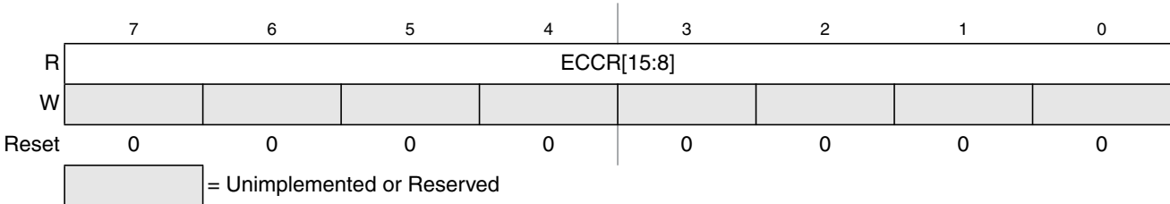
Figure 29-20. Flash ECC Error Results High Register (FECCRHI)
