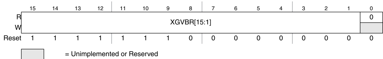
Figure 10-9. XGATE Vector Base Address Register (XGVBR)
