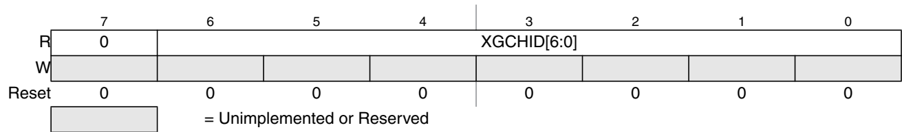
Figure 10-4. XGATE Channel ID Register (XGCHID)
