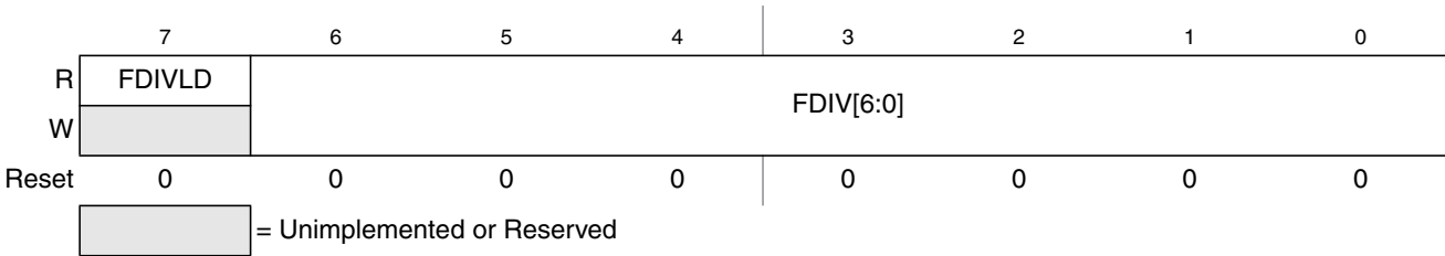
Figure 29-5. Flash Clock Divider Register (FCLKDIV)
