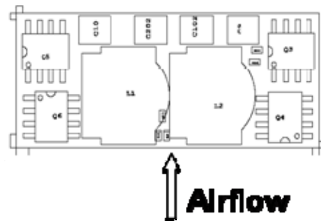
Figure 55. Airflow direction for thermal testing.
