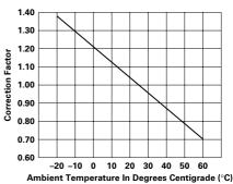
To use this chart: Read up from the ambient temperature to the curve, and across to find a correction factor. Multiply the breaker rating by the correction factor to determine the compensated rating. Calculate the overloads in terms of the compensated rating to use the published trip curve. Do not use these devices outside their specified operating temperature ranges.
