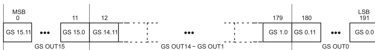
Figure 17. Grayscale Data Packet Format
