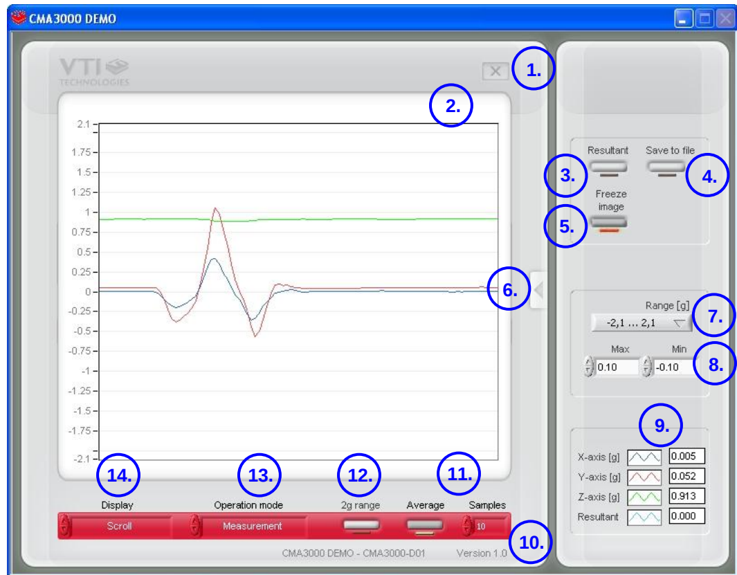
Figure 2. SCA3000 DEMO KIT Graphical User Interface
