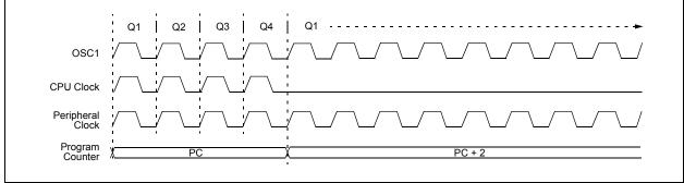
FIGURE 4-8: TRANSITION TIMING FOR WAKE FROM IDLE TO RUN MODE
