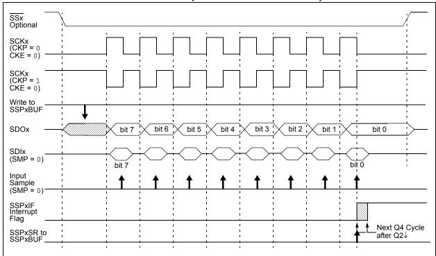
FIGURE 20-6: SPI MODE WAVEFORM (SLAVE MODE WITH CKE = 1)
