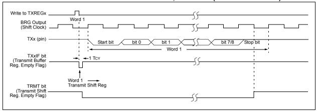
FIGURE 21-5: ASYNCHRONOUS TRANSMISSION (BACK-TO-BACK), TXCKP = 0 (TXx NOT INVERTED)
