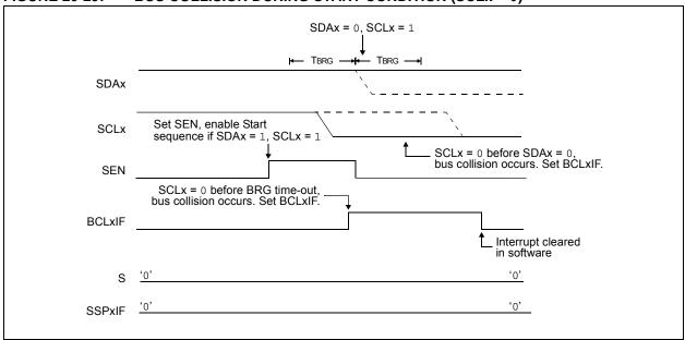
FIGURE 20-30: BRG RESET DUE TO SDAX ARBITRATION DURING START CONDITION
