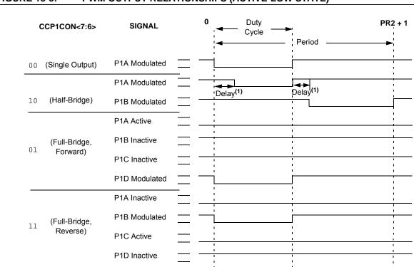
FIGURE 18-3: PWM OUTPUT RELATIONSHIPS (ACTIVE-LOW STATE)
