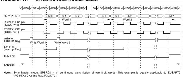
FIGURE 21-12: SYNCHRONOUS TRANSMISSION (THROUGH TXEN)
