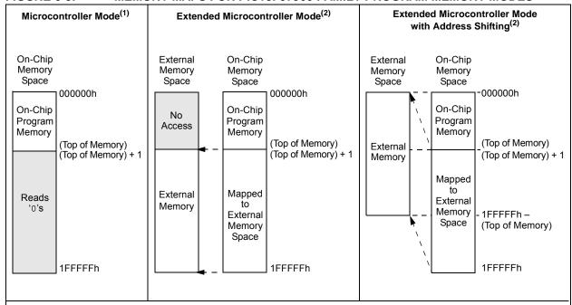
**Legend:** (Top of Memory) represents upper boundary of on-chip program memory space (see Figure 6-1 for device-specific values). Shaded areas represent unimplemented or inaccessible areas depending on the mode.
