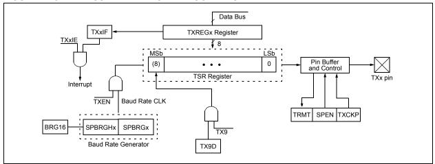
FIGURE 21-4: ASYNCHRONOUS TRANSMISSION, TXCKP = 0 (TXx NOT INVERTED)
