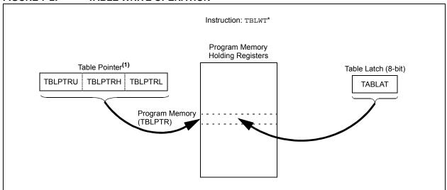
Note 1: The Table Pointer actually points to one of 64 holding registers, the address of which is determined by TBLPTRL<5:0>. The process for physically writing data to the program memory array is discussed in Section 7.5 "Writing to Flash Program Memory".
