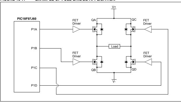
FIGURE 18-7: EXAMPLE OF FULL-BRIDGE APPLICATION
