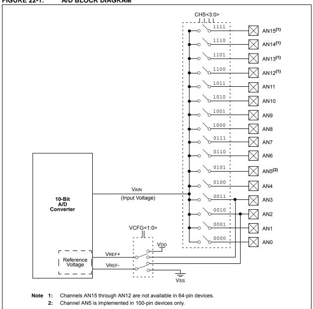
After the A/D module has been configured as desired, the selected channel must be acquired before the conversion is started. The analog input channels must have their corresponding TRIS bits selected as inputs. To determine acquisition time, see Section 22.1 "A/D Acquisition Requirements". After this acquisition time has elapsed, the A/D conversion can be started. An acquisition time can be programmed to occur between setting the GO/DONE bit and the actual start of the conversion.
