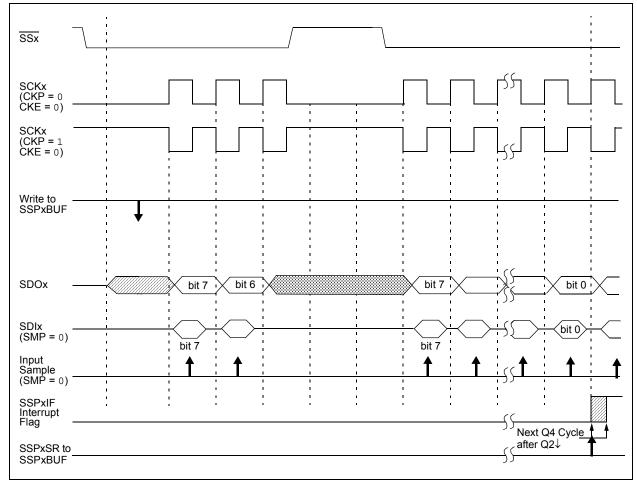
FIGURE 20-5: SPI MODE WAVEFORM (SLAVE MODE WITH CKE = 0)
