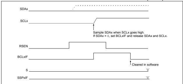
FIGURE 20-32: BUS COLLISION DURING REPEATED START CONDITION (CASE 2)
