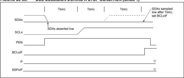
FIGURE 20-34: BUS COLLISION DURING A STOP CONDITION (CASE 2)
