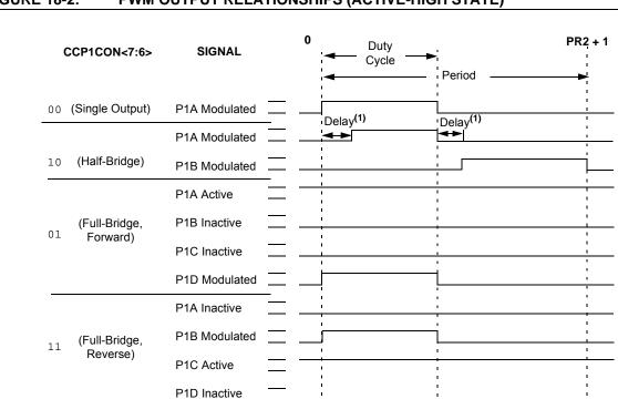
FIGURE 18-2: PWM OUTPUT RELATIONSHIPS (ACTIVE-HIGH STATE)
