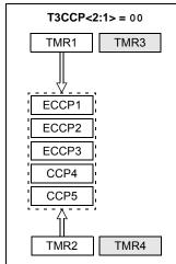
Timer1 is used for all Capture and Compare operations for all CCPx modules. Timer2 is used for PWM operations for all CCPx modules. Modules may share either timer resource as a common time base.
