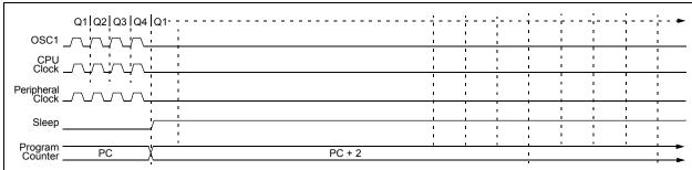
FIGURE 4-6: TRANSITION TIMING FOR WAKE FROM SLEEP MODE (HSPLL)
