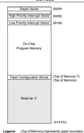
of on-chip program memory space (see Figure 6-1 for device-specific values). Shaded area represents unimplemented memory. Areas are not shown to scale.
