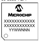
100-Lead TQFP (12x12x1 mm)
