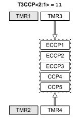
Timer3 is used for all Capture and Compare operations for all CCPx modules. Timer4 is used for PWM operations for all CCPx modules. Modules may share either timer resource as a common time base.
