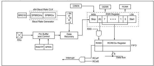
FIGURE 21-7: ASYNCHRONOUS RECEPTION, RXDTP = 0 (RXx NOT INVERTED)
