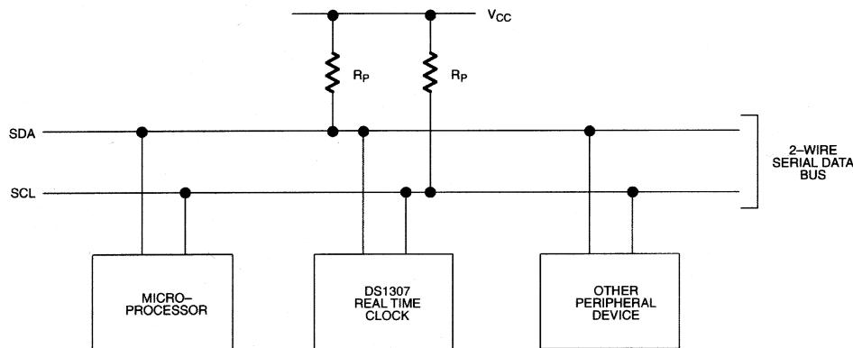
Figures 5, 6, and 7 detail how data is transferred on the 2-wire bus.
