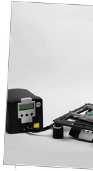
The MRS-1100A allows you the choice of using either the embedded profiling capability that can be configured to operate at a fixed temperature, or a four zone programming option. The unit also allows the temperature to be controlled either at the heat output (internal) or at the board (external). The “external” control function uses a thermocouple which can be placed on the board or a component.
