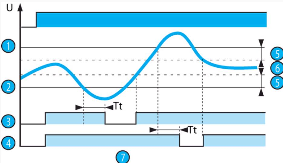
If the frequency of the controlled voltage exceeds the preset overfrequency threshold for longer than the time set on the front face (0.1 to 10 s), the corresponding output relay opens and its LED is extinguished. During the time delay, this LED flashes.
