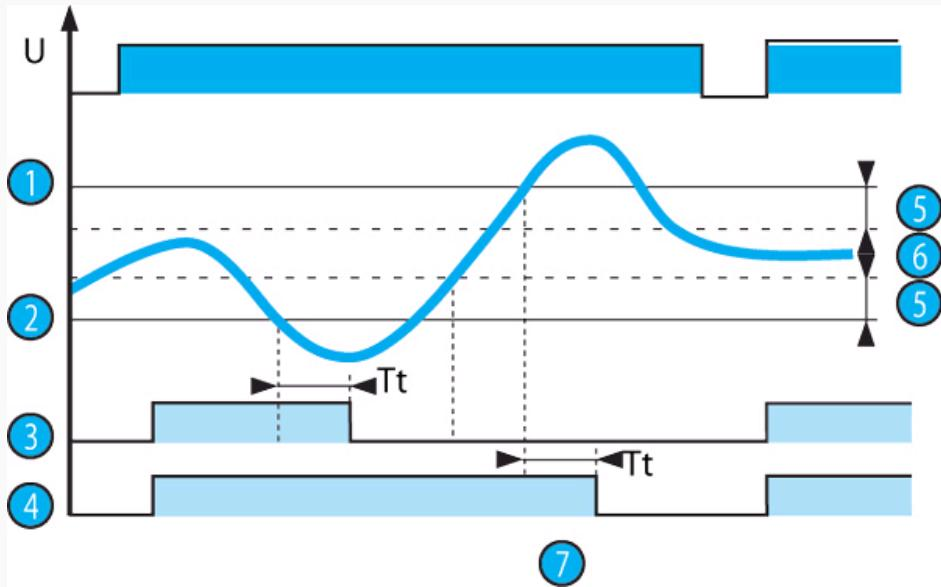
If "with memory" mode has been selected, the relay opens and stays in this position when threshold crossing is detected.
