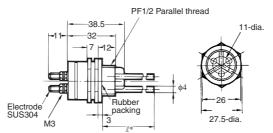
Standard holder construction includes three integral 300 mm length electrodes. However, a type having 1,000 mm length electrodes is available on request.
