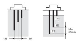
Electrodes are in actual contact with the liquid. Standard electrodes are made of stainless steel and usable in purified water, sea water, sewage, acid (except acetic acid, sulfuric acid, etc.) and alkaline liquids, although they may corrode depending upon the temperature and working conditions.
