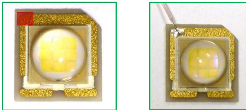
Figure 10. Thermal contact area highlighted in red (left) and example of TC probe attachment (right).
