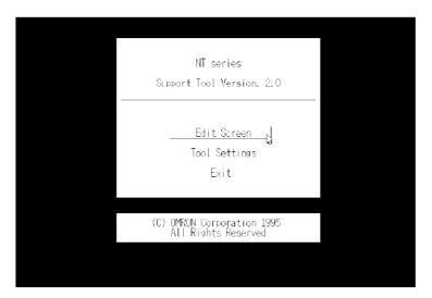
**Reference:** When the support tool is started up for the first time, the "Tool Settings" screen is displayed first. See 3-3 "Tool Settings" Screen (p.22).
