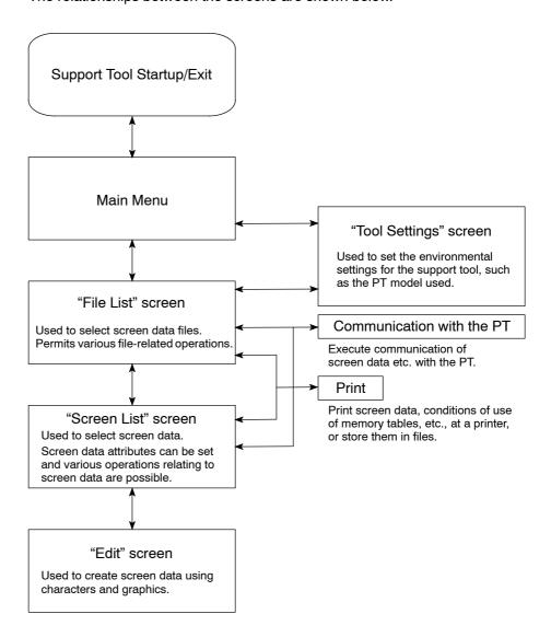
**Reference:** When the support tool is started up for the first time, the "Tool Settings" screen is displayed first.
