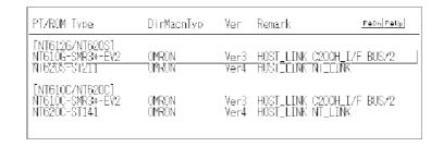
When the window is displayed by pressing [F1] (TypSel), the bar cursor is located at the PT model which was set for "PT Type".
