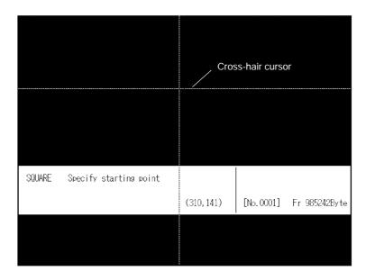
When the cross-hair cursor touches the menu box, the menu box is automatically cleared from the screen and coordinates are displayed at the top right of the screen. When the operation with the cross-hair cursor is completed, the menu box is redisplayed.
