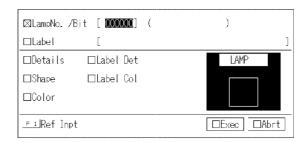
S LampNo. /Bit: If direct connection is not used, set the lamp number here. If direct connection is used, set the bit (lamp bit) allocated at the PC.
