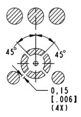
RECOMMENDED SOLDER STENCIL (REFER TO LAND PATTERN DETAIL FOR DIMENSIONS NOT SHOWN)
