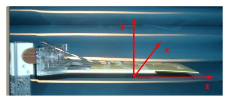
FXP831 on Baxter device to indicate the testing coordinate
