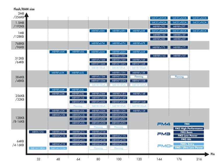
The Cypress FM MCU lineup consists of three families—FMO+, FM3 and FM4—each of which uses a specific ARM Cortex-M core. Users can easily transition between device types and families because of the compatibility of the instruction sets.
