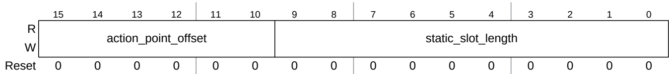
Figure 13-65. Protocol Configuration Register 0 (PCR0)
