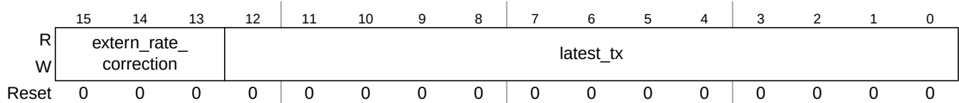
Figure 13-86. Protocol Configuration Register 21 (PCR21)
