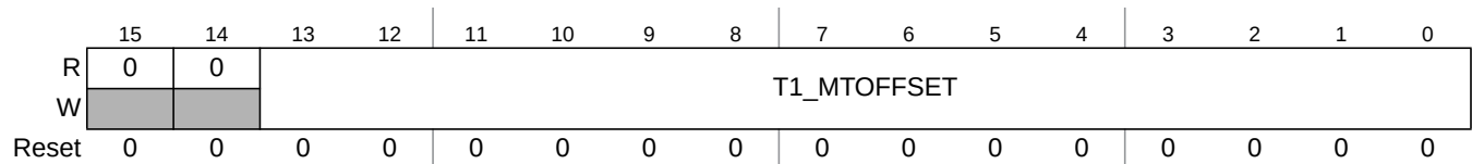
Figure 13-42. Timer 1 Macrotick Offset Register (T1MTOR)
