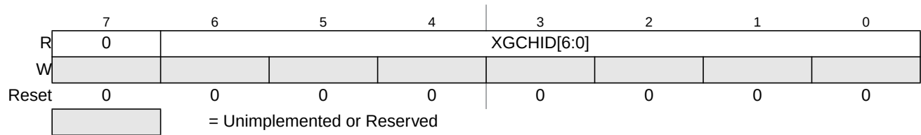
Figure 14-4. XGATE Channel ID Register (XGCHID)
