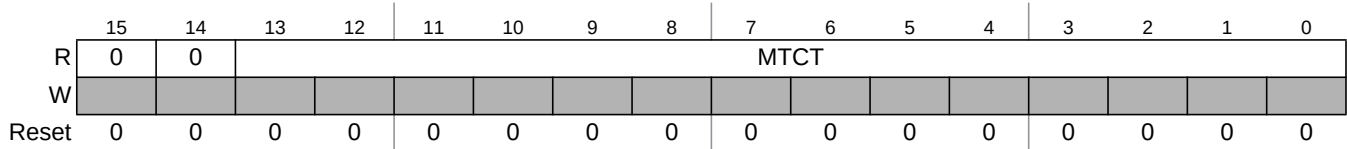
Figure 13-24. Macrotick Counter Register (MTCTR)
