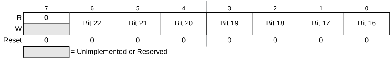
Figure 16-15. Debug Comparator Address High Register (DBGXAH)
