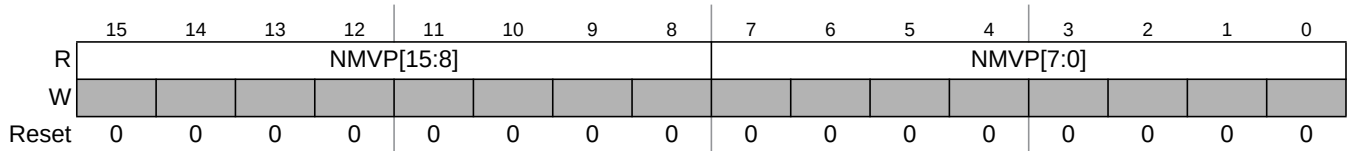
Figure 13-38. Network Management Vector Registers (NMVR0–NMVR5)
