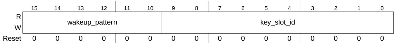
Figure 13-83. Protocol Configuration Register 18 (PCR18)
