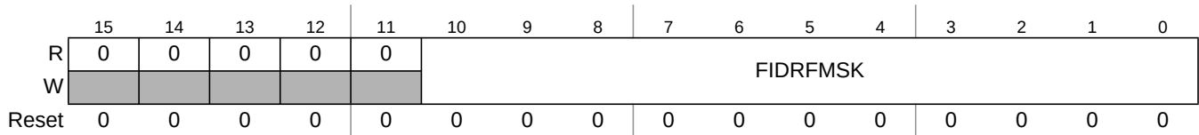
Figure 13-60. Receive FIFO Frame ID Rejection Filter Mask Register (RFFIDRFMR)
