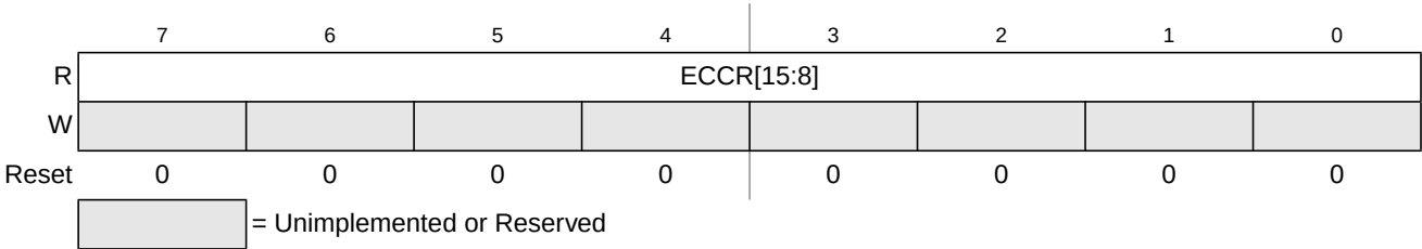
Figure 8-20. Flash ECC Error Results High Register (FECCRHI)
