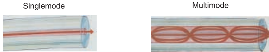
Figure 2. Singlemode and Multimode Fibers
