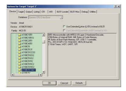
If the device is not listed in your KEIL μvision release, select another Atmel MCU: AT89C51RD2/ED2 for AT89C51RE2 and AT89C51SND1 for AT85C51SND3x. ■ To download the application code into the target, use the "Load button":
