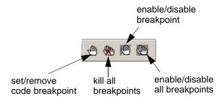
Code breakpoints can be either hardware breakpoints (addresses comparators) or software breakpoints (1-byte TRAP instruction executed in place of existing opcode).
