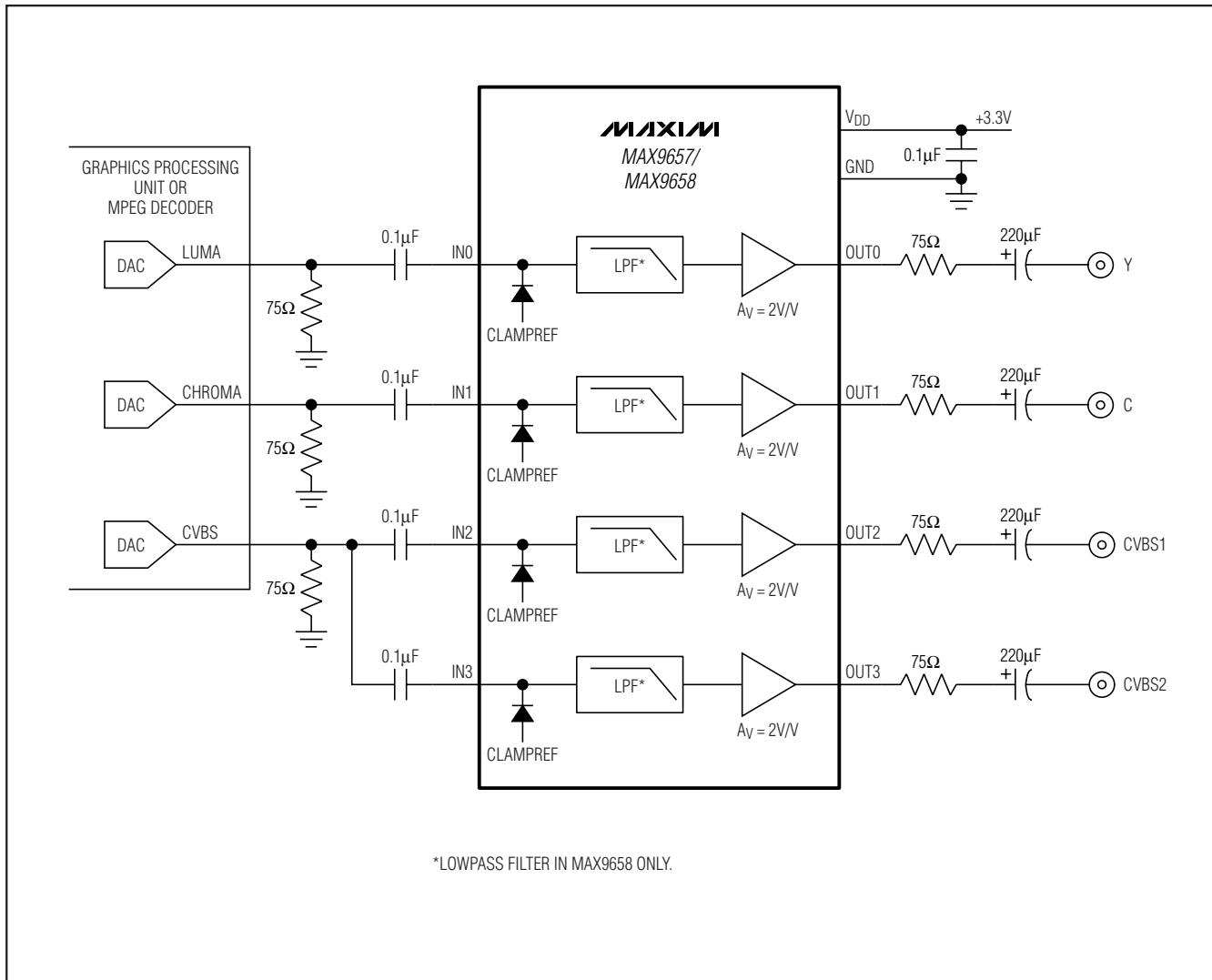
Figure 1. AC-Coupled Outputs
