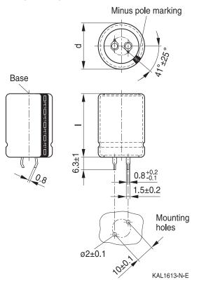
Snap-in terminals, length  $(6.3\pm1)$  mm. Also available in a shorter version with a length of (4.5-1) mm. PET insulation is marked with "PET" on the sleeve. Safety vent on the case wall.
