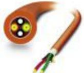
rugged GOF installation cable for inner areas with highly tear-proof aramid strain-relief elements. Individual elements consist of highly flexible FRNC material. The cable is halogen-free, ozone and UV resistant and has a rugged polyurethane (PUR) outer sheath.
