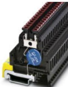
Modular terminal block with varistor as surge voltage protection between clamping connector and DIN rail, separate ground connection, nominal voltage: 60 V AC, mounting on NS 35/7.5, terminal width: 6.2 mm, terminal height: 69 mm
