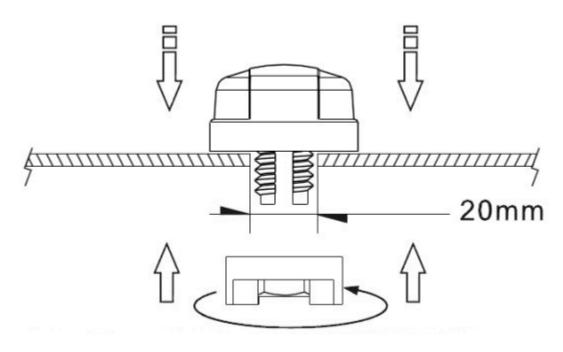
Recommended torque for mounting is 24.5N·m Maximum torque for mounting is 29.4N·m
