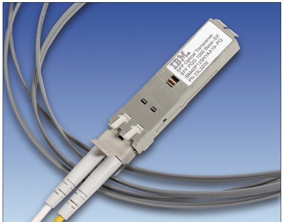
Small Form Factor transceiver (SFP) with LC connector fiber cable
