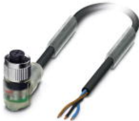
Sensor/Actuator cable, 3-position, PUR halogen-free, Black-gray RAL 7021, Free cable end, with 2 LEDs, PIN 2+4 bridged, on Socket angled M12, A-coded, with 2 LEDs, PIN 2+4 bridged, Cable length: 3 m
