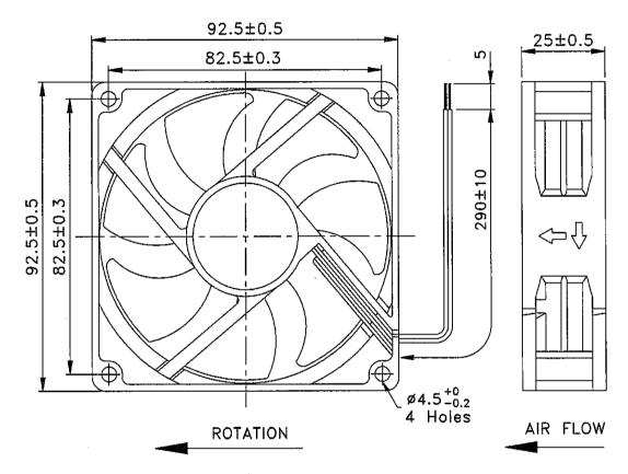
LEAD WIRES: UL 1007, AWG24, L = 290 +/- 10 MM Red = positive; Black = negative.
