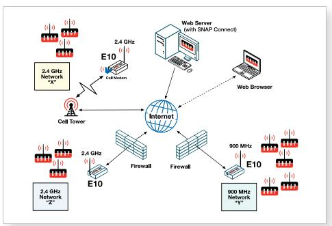
The **SNAP CONNECT E10 APPLIANCE** connects SNAP networks to the Internet using built-in Ethernet or USB Cell modem or Wi-Fi adapter. Shown here, the web browser can monitor and control three remote SNAP networks in real time.
