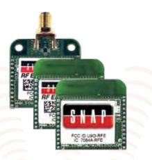
Synapse provides reliable RF Engines® that support a range of frequencies and bandwidths. These small, low-power, transceiver modules, running from sub-GHz to 2.4GHz, have a long range and the lowest power consumption in the industry.
