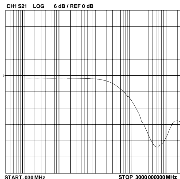
Figure 2 - Typical Insertion Loss S21
