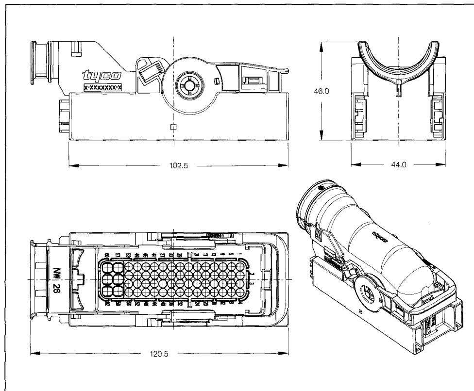
Sealed Receptacle Housings for Mixed 1.5 and 2.8 Contacts
