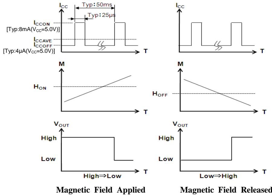
3-5 Electric Characteristics/ Absolute Maximum Rating ( $T_a=+25^\circ C$   $V_{CC}=5.0V$ )
