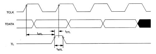
NOTE: The rising edge of TL causes the internal pattern generation circuitry to be reloaded; the first bit of the new pattern (the shaded one) will appear after two TCLK periods.
