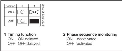
DIP switch functions CM-MPS.x1
