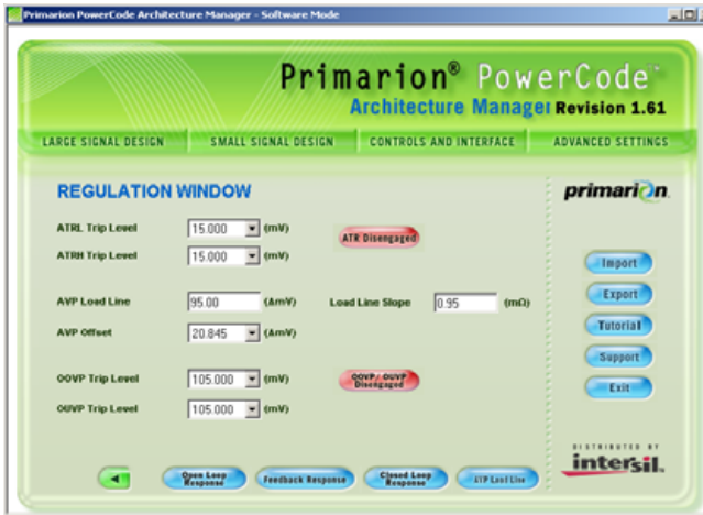
FIGURE 23. PRIMARION POWERCODE LOADLINE AND ATR SETTINGS
