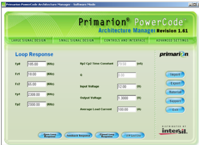
FIGURE 24. PRIMARION POWERCODE LOOP RESPONSE SETTINGS
