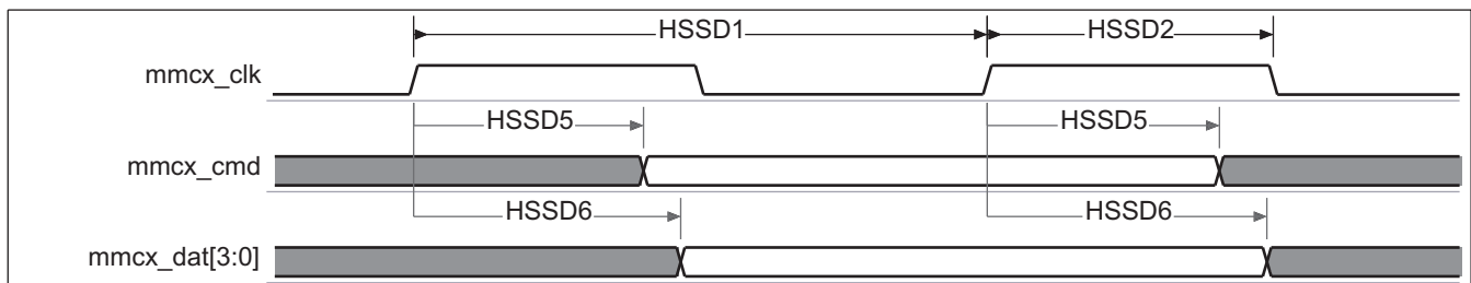
Figure 6-65. MMC/SD/SDIO – High-Speed SD Mode – Data/Command Receive
