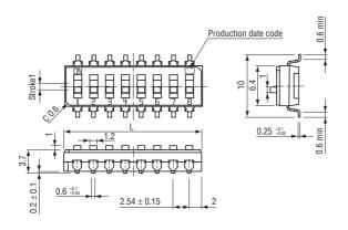
Convex knob of 1 mm, Through hole pin
