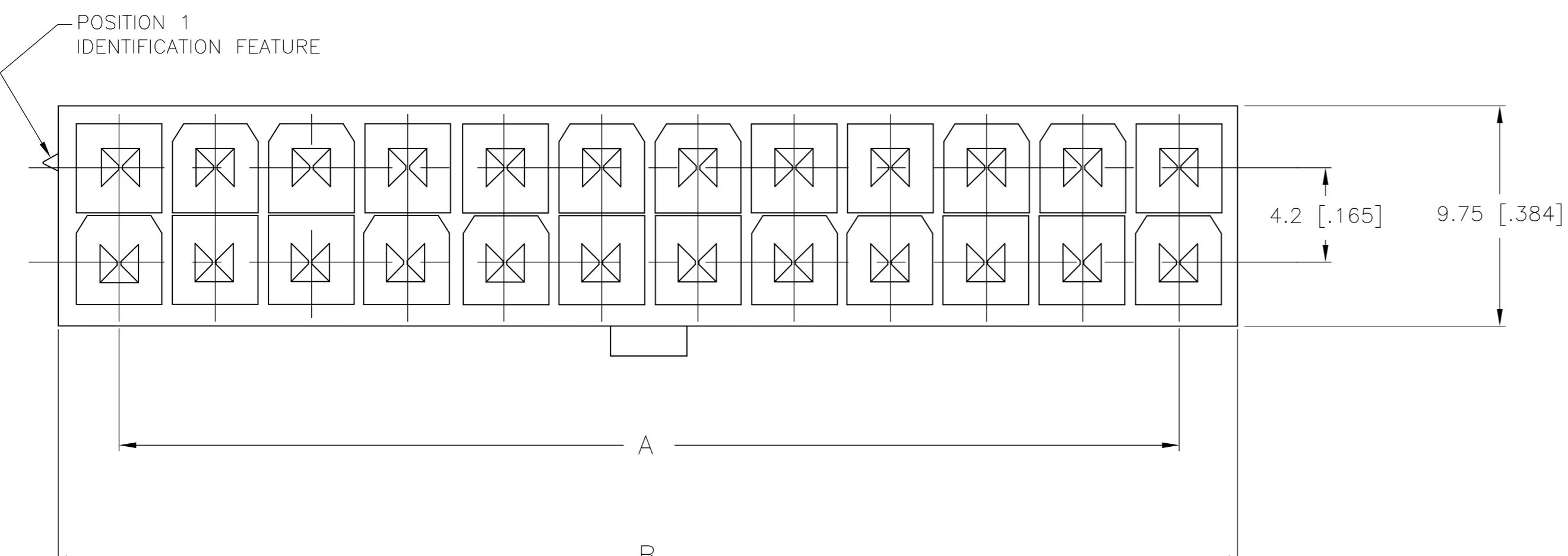
1 MATERIAL: HOUSING: NYLON, UL94V-0
