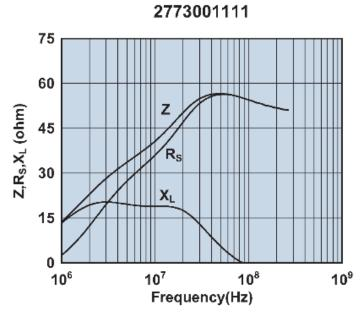
Impedance, reactance, and resistance vs. frequency.
