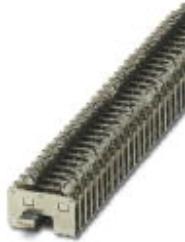
Power terminal block, Connection method Screw connection, Load current : 76 A, Cross section: 0.5 mm 2 - 16 mm 2 , Width: 8 mm, Color: aluminum
