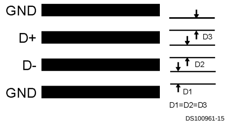
FIGURE 6. Recommended Diode Trace Layout
