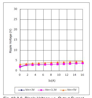
Fig. 12-3-6. Ripple Voltage v.s. Output Current
