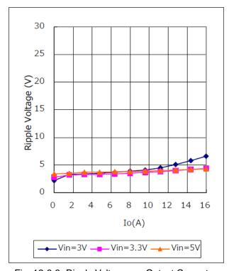
Fig. 12-3-3. Ripple Voltage v.s. Output Current
