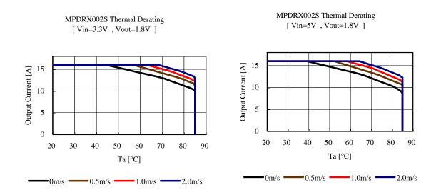
The above derating limits apply to this product soldered directly to 101.6\*180mm\*1.6mm PCB (double-sided, with 70um copper). Any adjacent parts of high temperature may cause overheating. For reliable operation, please ensure that the FET temperature of this product is maintained below 120°C and the inductor temperature is below 106°C.
