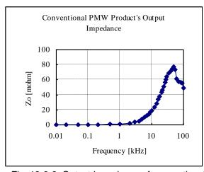
Fig. 12-2-2. Output Impedance of conventional product
