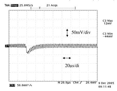
Fig. 12-1. Load Transient Response
