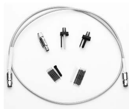
Figure 3.14. Agilent 54006A for probing high frequency, up to 100 \Omega impedance signals.
